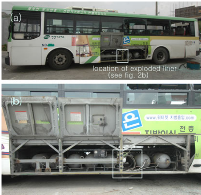
FIG. 2—The location of liners. The bus had a total of eight liners that were tied with parallel pipe lines. The liner that was the sixth from the front side of the bus had exploded.
