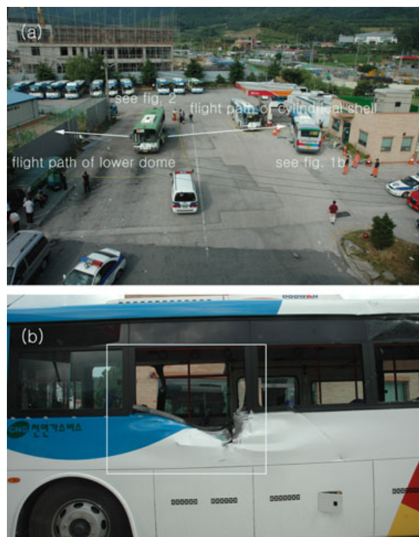
FIG. 1—(a) The gas station where the accident took place. Arrows indicate the flight path of a cylindrical shell and a lower dome. (b) The damage to the bus that was parked beside the bus that featured the explosion. The quadrangle indicates the trace where the cylindrical shell went through this adjacent bus.
